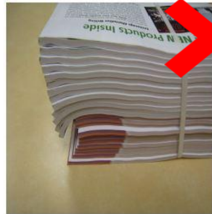
DAMAGE CAUSED BY DOUBLESTRAPPING
